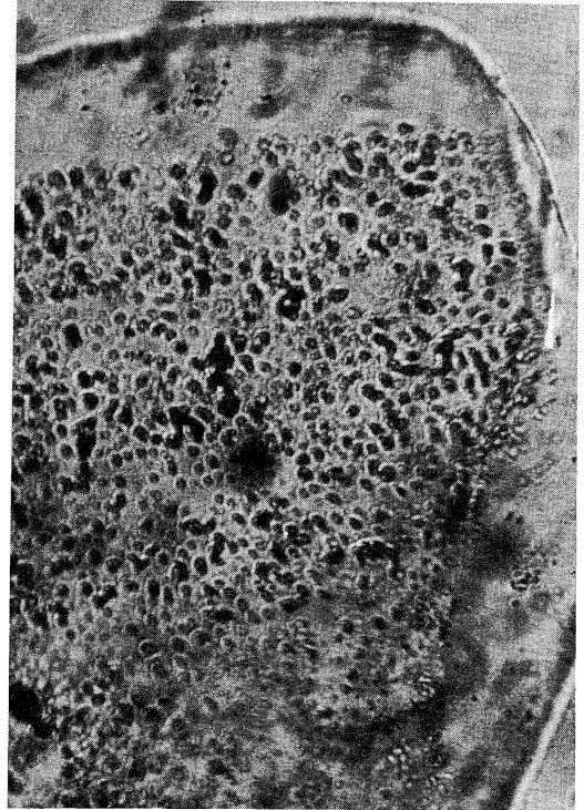
Fig. 1. - Fluid inclusions concentrate in the central area, X 50.
