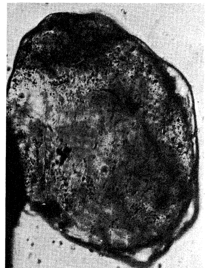
Fig. 4. - Secondary overgrowth on quartz, X 50.
