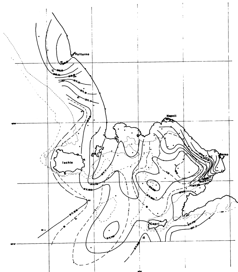
Figure 1 - Salinity (S‰ ,full lines) and depth (metres, dotted lines) of the homogeneous surface layer in the Gulf of Naples.
