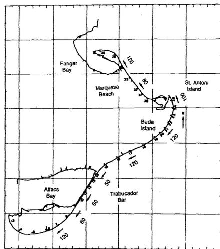
Figure 1. Net longshore transport rates in the Ebro Delta (transport in thousands of cubic meter per year)(modified from Jiménez *et al.* 1992)
