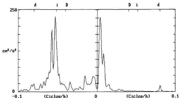
Rotary spectrum (negative frequencies correspond to the clockwise rotation) at 115 m. depth.
