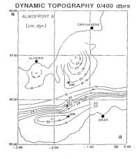
Fig 2.- Results from the 83 stations of synoptic survey: Dynamic topography of the surface level relative to the 400 surface level relative to the 400 dbars level. The south position of the jet and two eddies at north are clearly shown. The stars indicate the positions of the 3 THES stations which will presented to evidence the subduction of the water, North of the jet front, Southward and helow southward and below the core of the jet.
