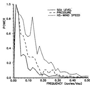
FIG.2 Normalized power spectrum of pressure, sea level and NS-wind component. The normalizing factors are respectively: 865.6 cm<sup>2</sup>, 752.8 mbar<sup>2</sup>, 448.6 (m/sec)<sup>2</sup>
