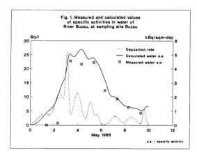
The main processes governing the shape of the peak in water specific activity are radionuclide accumulation vs. decay and longitudinal transport.
