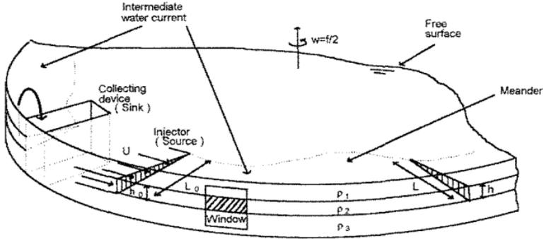
Fig. 1. Sketch of the experimental facility
