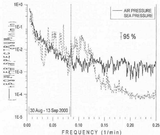
Figure 1: Power spectra of the air and sea pressure measured on the MedGLOSS tide gauge.
