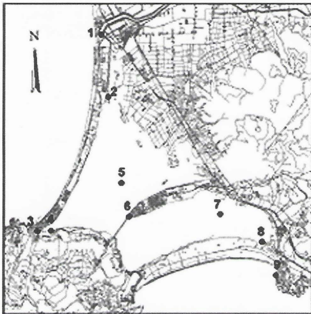
Fig. 1. Position of the gauges. 1-4-6-9 Hydro-meter; 2-3-8 Hydro-meter; current-meter; multi-parametric gauge, 5-7 Hydro-meter; current-meter; multi-parametric gauge; wind-meter.
