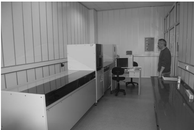
Fig. 1. EMCOL's ITRAX core scanner does XRF analysis, digital radiography and colour scanning of sediment cores at sub-mm scale resolution.
