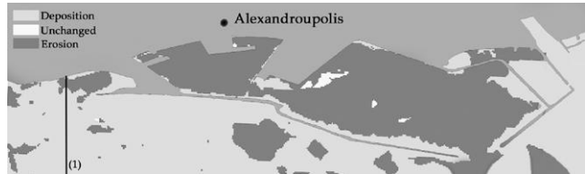
Fig. 1. Bathymetric changes, after the comparison of the bathymetric charts of 1960 and 2004. (1): Position of bathymetric profiles (figure 2).
