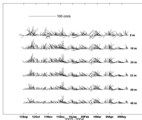
Fig. 1. Stick diagram of daily mean currents at each depth.
