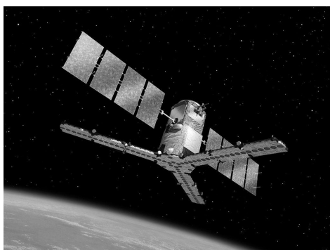
Fig. 1. The 69 antennas along the SMOS arms (by P. Carril for ESA)
