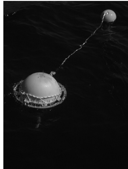
Fig. 2. Preliminary prototype of the drifting buoy with an additional flotation in the line that connects to the standard cylindrical drogue
