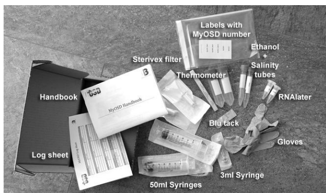
Fig. 1. Content of the MyOSD sampling kit. Each kit had a unique MyOSD number to keep better track of the collected sample and its contextual data.
