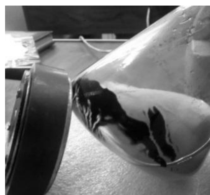
Fig. 2. Collecting coated cells suspension by application of external magnetic field.
