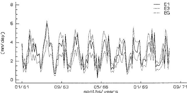
Figure 1. Mean monthly evaporation (mm/day) calculated using three different formulas for station Trieste, period 1961-1970. Time series denoted as E1 is calculated using Jacobs formula, E3 using Laevastu and EG using Gills formula.
