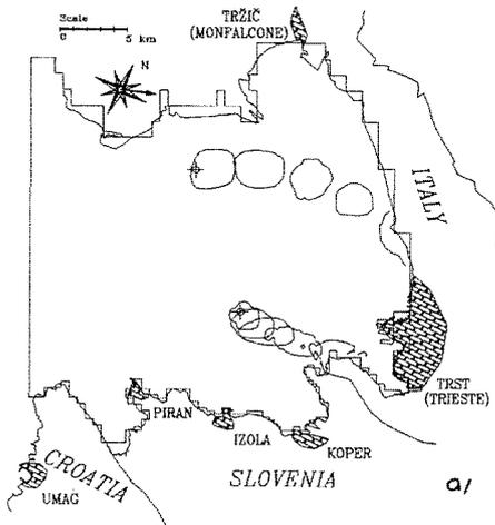
Fig. 1. Simulation of oil spreading for spill at two locations in the Gulf of Trieste with a WSW wind of 8 m/s. Oil slicks in 4, 10, 18, 28 and 40 hours after the spill of 75 tons of diesel fuel.
