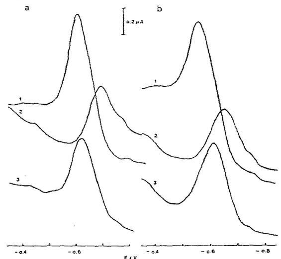
Fig. 2. (a) A.c. voltammograms of  $10^{-4}$  M ONP in 0.5 M NaCl, pH 8.4; without SAS, acc. time 180 s (curve 1); in the presence of 1 mg/l albumine, acc. time 180 s (curve 2) and 1 mg/l humic acid, acc. time 60 s (curve 3). (b) A.c. voltammograms of  $10^{-4}$  M ONP in seawater samples, Station 107, 0.5 m, May 17, 1994 (curves 1 and 3), Station 105, 0.5 m, May 17, 1994 (curve 2). Acc. time (1) 0, (2) and (3) 180 s.
