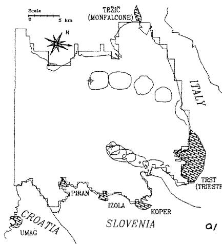
**Fig. 1.** Simulation of oil spreading for spill at two locations in the Gulf of Trieste with a WSW wind of 8 m/s. Oil slicks in 4, 10, 18, 28 and 40 hours after the spill of 75 tons of diesel fuel.
