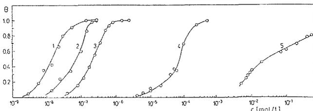
Figure 1. The adsorption isotherms of different polyacrylic acids in 0.55 M NaCl, pH 1.8. (1) PAA MW = 90000, (2) MW = 5000 (3) MW = 2000 and (4) acrylic acid and (5) glutaric acid. Adsorption time  $t = 60$  s, potential  $E = -0.6$  V vs Ag/AgCl reference electrode.  $\theta =$  degree of surface coverage.
