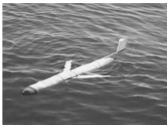
Fig. 3. (See page 109 for original color plate) Slocum glider (Webb Research).
