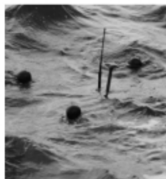
Fig. 1. (Top) Photograph of a CODE drifter showing the GPS (left) and Argos (right) antennas at the top, and the main structure of the drifter with 1-m height sails. (Bottom) CODE drifter floating at the sea surface.
