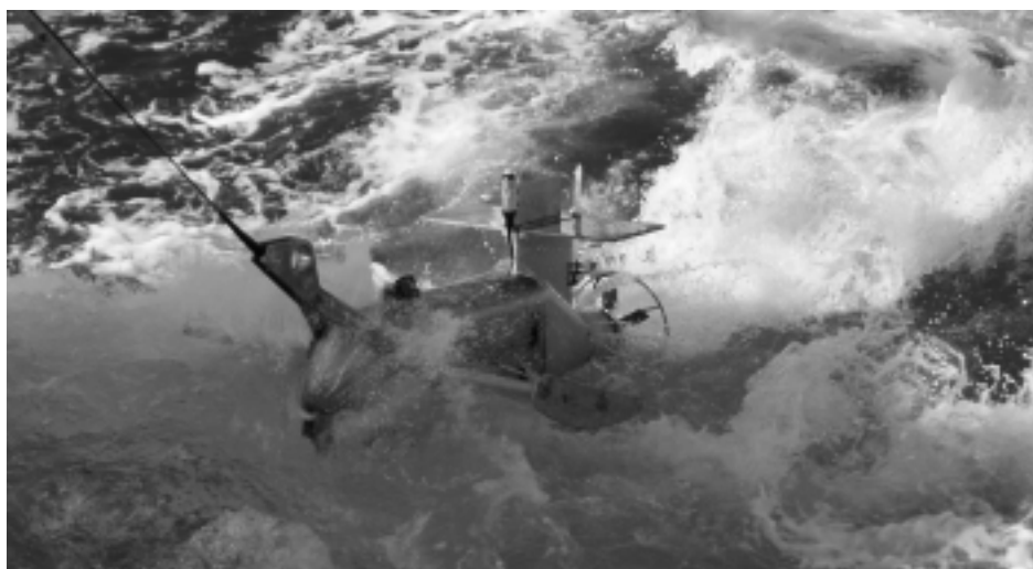
Fig. 4. (See page 109 for original color plate) The SeaSoar vehicle at the surface awaiting recovery. Photograph courtesy of Prof. R.T. Pollard, National Oceanography Centre, Southampton, U.K.
