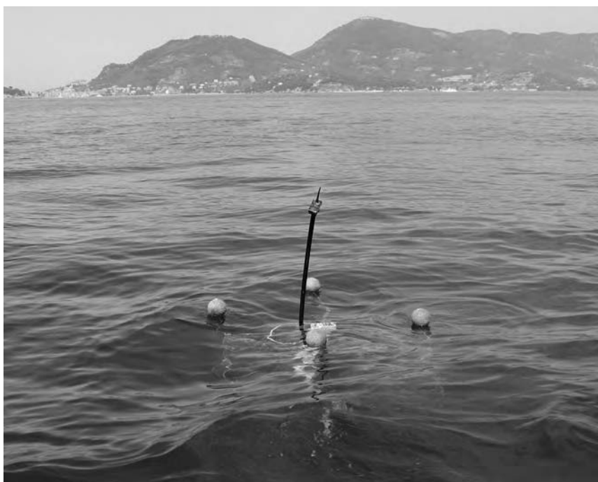
Fig. 1. Photograph of a CODE drifter in the Gulf of La Spezia. Only the GPS and GSM/GPRS antenna and four small spherical floating balls protrude above the sea surface.
