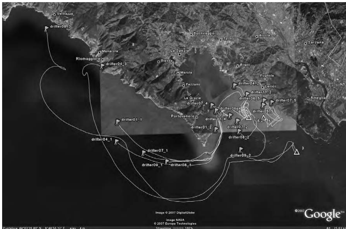
Fig. 4. Edited and smoothed (15-min running average) trajectories of the drifters deployed in the Gulf of La Spezia in June 2007. The diversity of drifter motions within the Gulf is evident. The drifters that eventually moved out of the Gulf on its western flank were entrained to the northwest with the strong coastal currents. Triangles indicate the deployment locations, whereas the last fixes are shown with flags.
