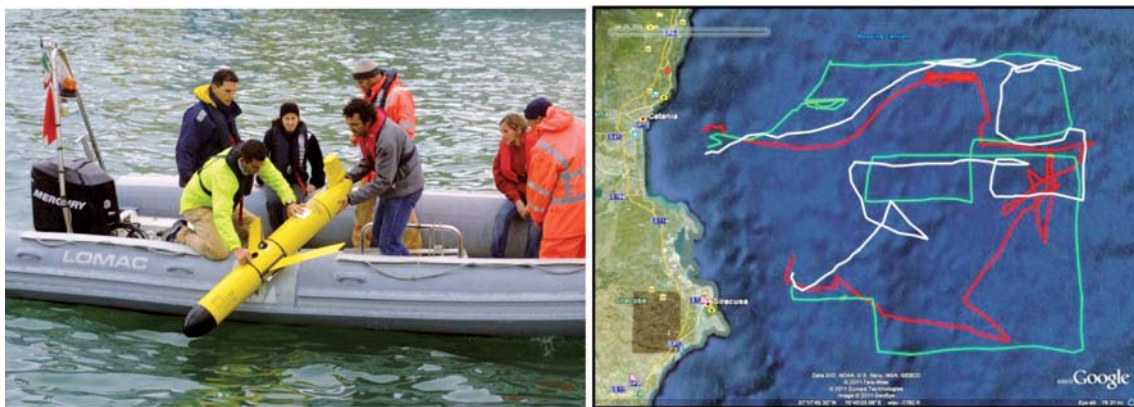
Fig. 2. Left: illustration of a glider deployment phase. Right: 3 glider simultaneous tracks showing regular transects and adaptive sampling phases.
