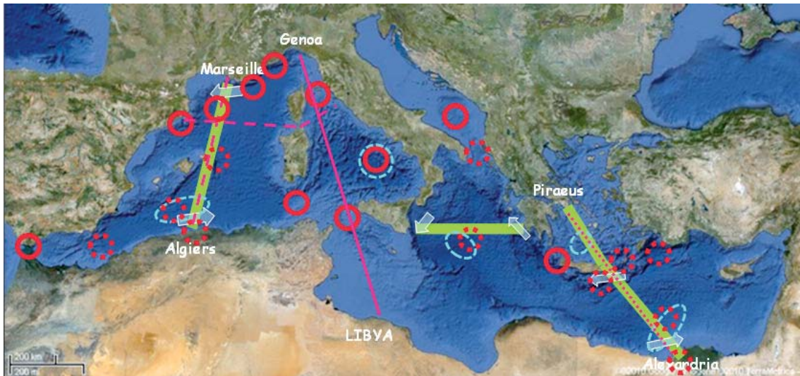
Figure 5. Suggested backbone for a Med-SHIP program (thick transects), and synergy with the monitoring programs HydroChanges (circles: existing stations, dotted circles: suggested complementary stations), and Transmed (thin transects; plain: existing, dashed: completion planned before late 2012; dotted: suggested). The arrows represent the local general circulation. The dashed ellipses represent the deepest areas.
