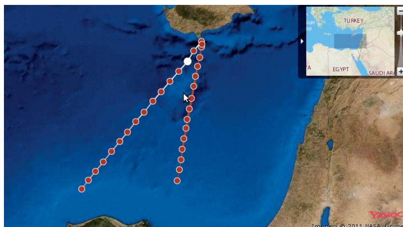
Fig. 3. Map of Expendable Bathythermograph (XBT) repeat lines carried out by the Oceanography Center, University of Cyprus. During the most intensive sampling period, temperature profiles were collected down to 800 m every 10 nautical miles along one of these lines monthly from May 2004 to October 2005.
